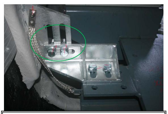
Figure 34 Left rear nacelle attachment. Bolting moved on nacelle end of connector.
