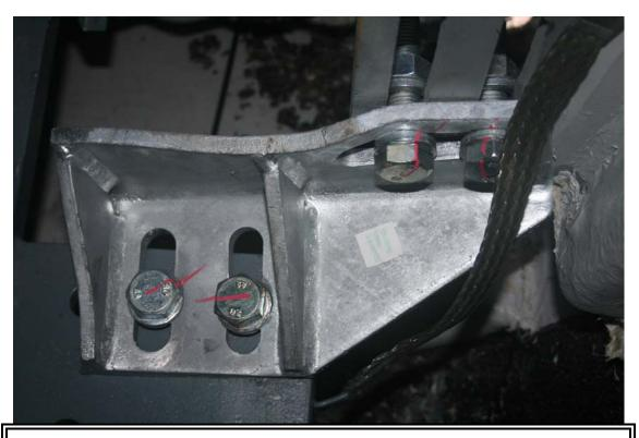
Figure 42 Right rear nacelle attachment. Connector bent. Nacelle bracket bolting moved.
