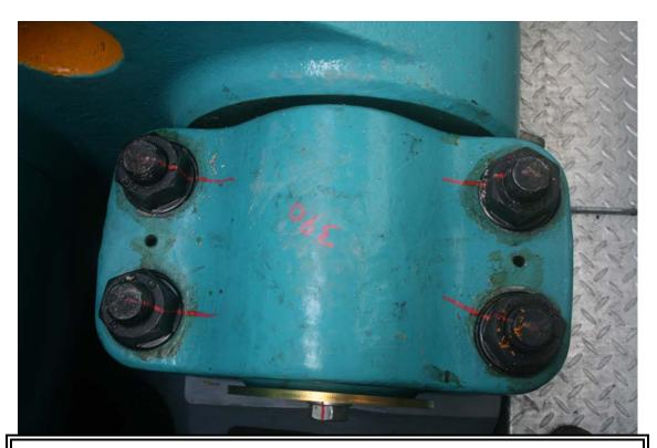
Figure 49 Right rear gearbox mount bolting. Typical of right front gearbox bolting.
