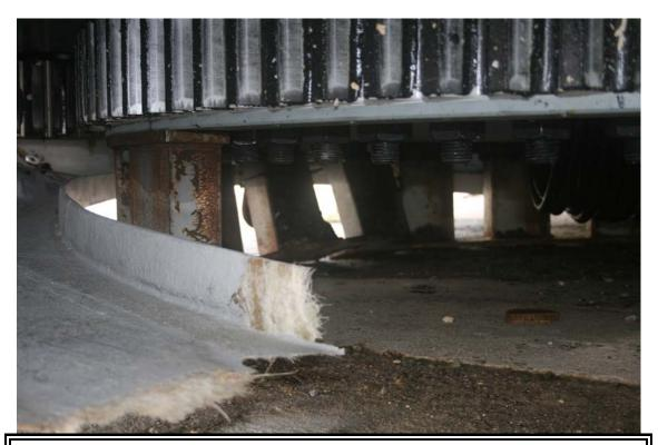
Figure 24 Bent shipping legs attached to the yaw gear.
