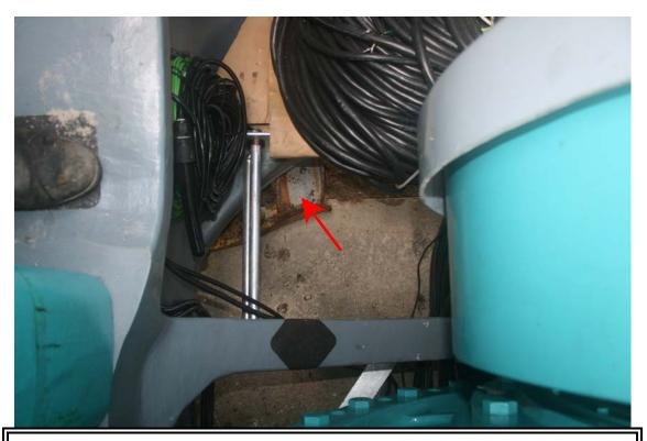
Figure 22 Tower cables coiled below main shaft. Bent shipping legs at arrow.
