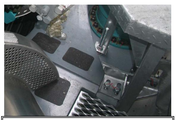
Figure 48 Right center nacelle attachment. Connector bent. Nacelle bracket bolting moved.
