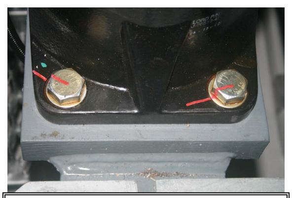
Figure 36 Left front generator mount. Generator frame attachment bolting not moved.
