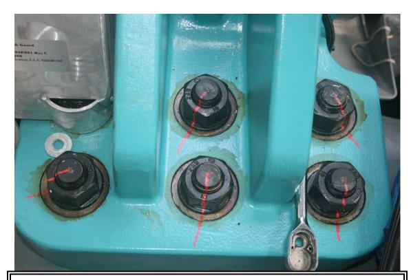
Figure 19 Close-up view of main pillow block bearing left side bolting.
