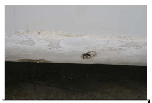
Figure 9 Penetration in nacelle near the right rear.
