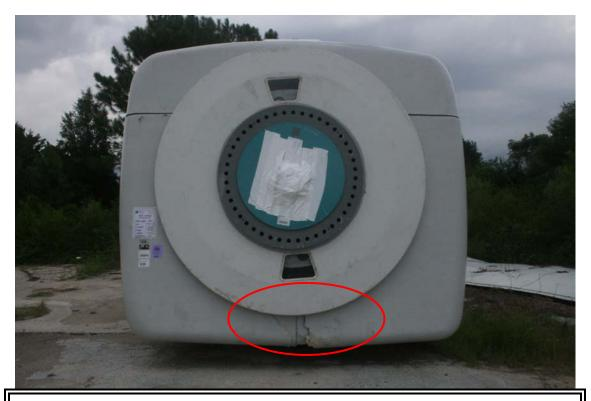
Figure 6 Front of machine head; nacelle fractured at bottom center.
