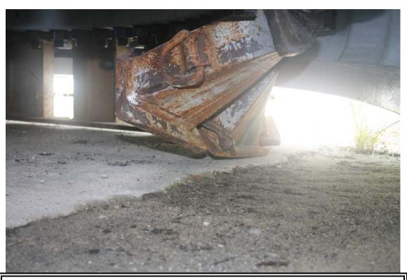
Figure 25 Bent shipping legs attached to the yaw gear.
