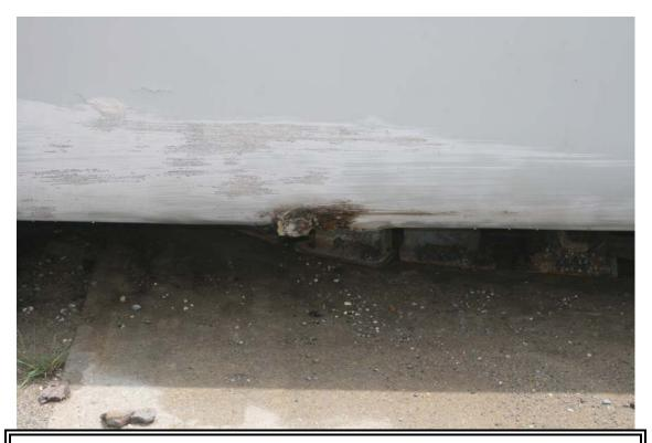
Figure 10 Penetration in nacelle right side near the center.
