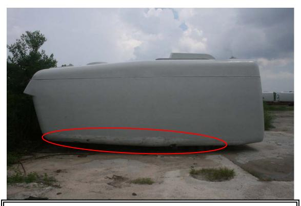
Figure 8 Right side of machine head with nacelle scrape marks and penetrations.
